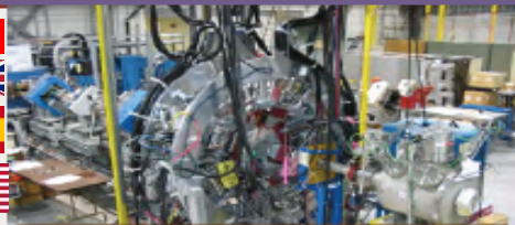
TIGRESS in-beam gamma-ray spectrometer
